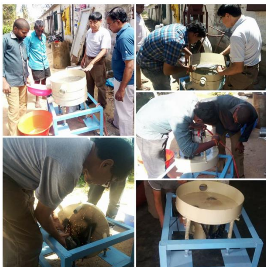
Testing of Vibro grader
