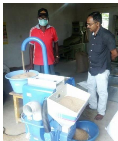
Trials with Otake rice huller
