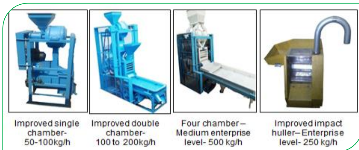
Figure 1: Improved impact hullers for processing small millets developed in the project
