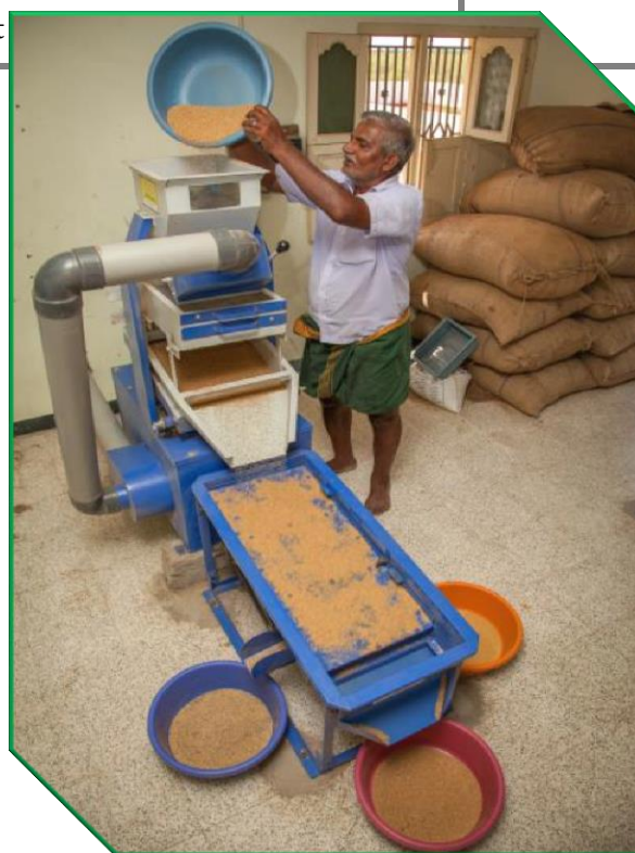
Figure 22: Small millet processing unit set up by Peraiyur FPO
