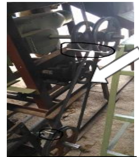
Fig. 7: Large overhang load on pillow block
