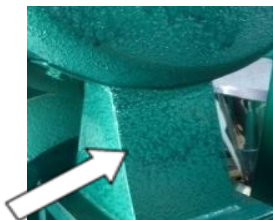
Fig. 15: Pyramidal outlet is better suited
