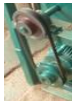
Fig. 22: Avoid power transfer from larger to smaller
