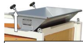
Fig. 29: Hopper with two control valves
