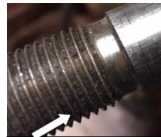
Fig. 14: Threads in need of rounding off
