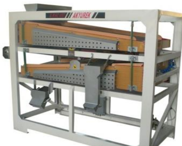
Fig. 9: Grader with sieve decks organised in a zigzag manner
