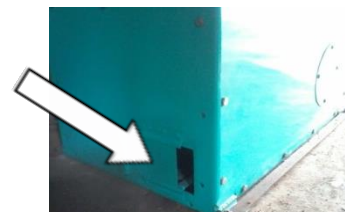
Fig. 11: Provision for cleaning
