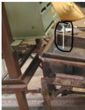
Fig. 3. The level of drop when grains move from aspirator to grader
