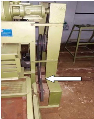
Fig. 26: Reducing the space between the main frame and safety guard
