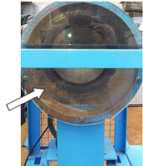
Fig. 23: Stagnation observed in impeller chamber
