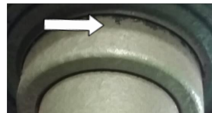
Fig. 18: Molten grease in the bearing
