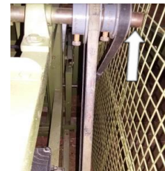
Fig. 27: Reduce the length of shaft
