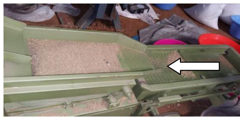
Fig.4: Chute design need to be modified
