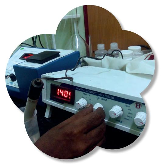
Apparatus for conductivity test
